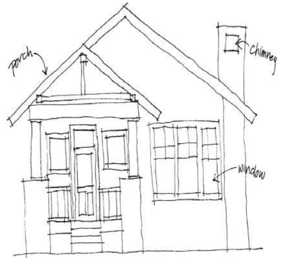
Inappropriate Drawing: Scale and character are not clearly conveyed. Dimensions are missing.
